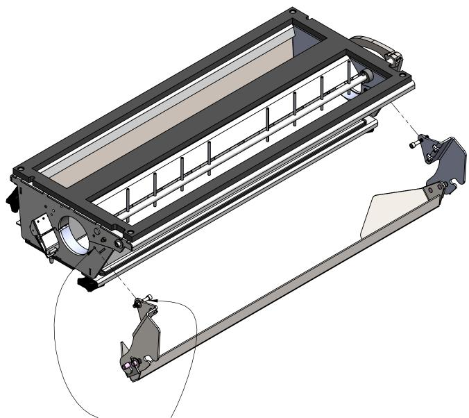
Remove bolt at both ends of meter housing. Insert bolt included with drain chute from inside, through meter wall and drain chute bracket. Tighten flange nut on outside.
